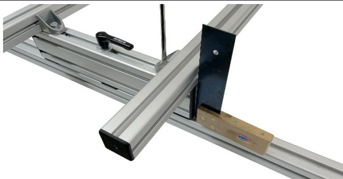
Figure 71: Cross rails flush with the supports on the longitudinal rails
