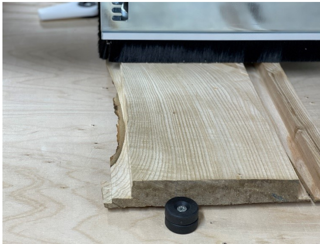
Figure 96: Machining the left edge of the board
