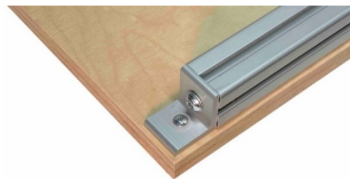
Figure 75: Fastening the right longitudinal rail to the worktop
