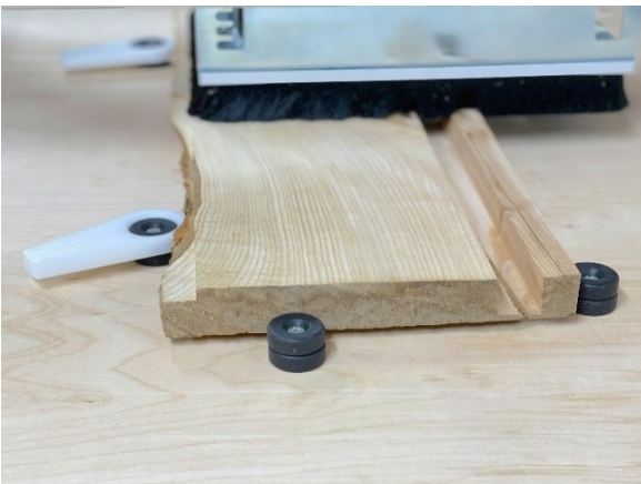
Figure 100: Grooving width 23 mm
