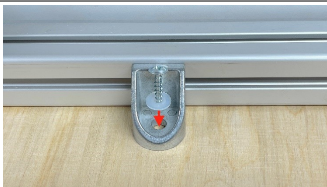
Figure 84: Fastening the longitudinal rails
