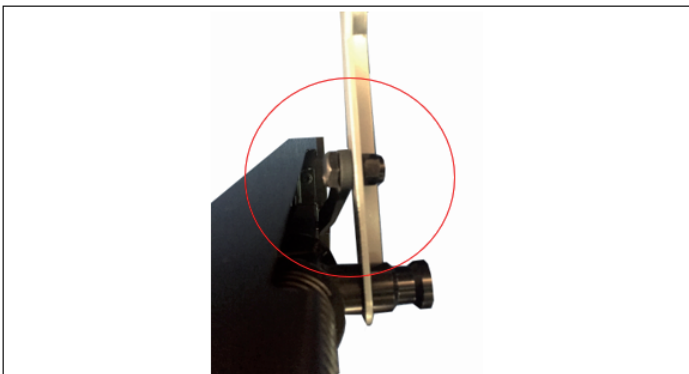
Step 17. Attach the crossbar to the drum lid and tighten using the two bolts removed in the previous step. It does not matter which position you
