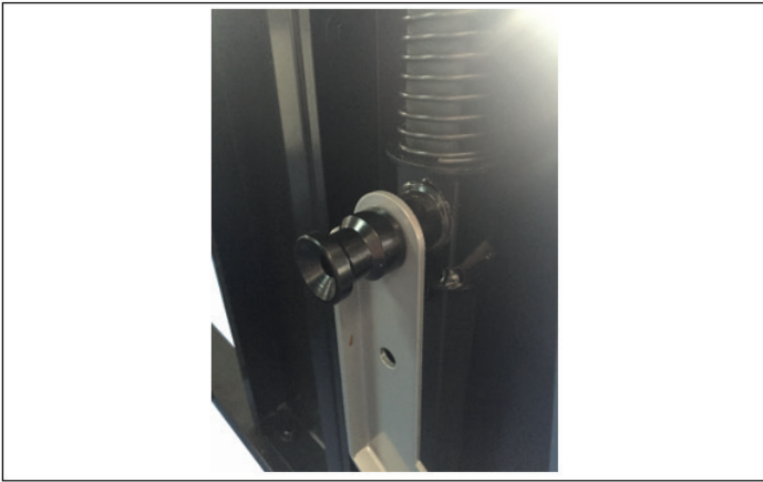
Step 14: Secure the topping with (2) M8 x 30mm hex bolts.
