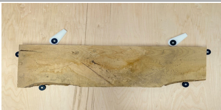
Figure 89: Fixing a wooden board to the work plate (as an example)
