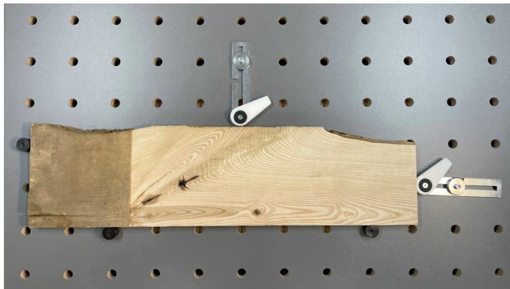
Figure 90: Fastening a wooden board to the hole matrix board
