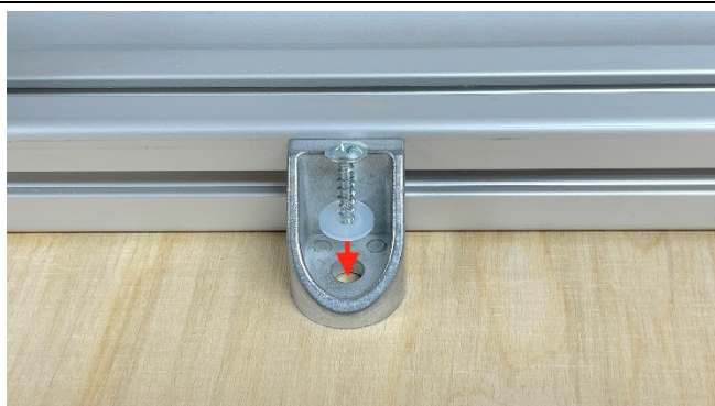
Figure 84: Fastening the longitudinal rails
