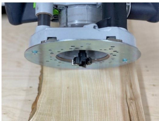
Figure 95: router bit for flattening
