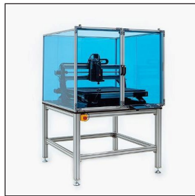
Available in three sizes - up to 1030 x 1030mm working area to mill wood, aluminum, plastic and fiberboards
